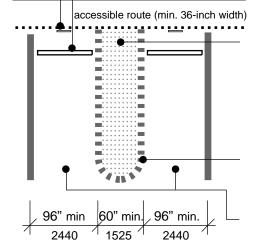
Access aisle of at least 60-inch width must be level (1:50 maximum slope in all directions), be the same length as the adjacent parking space(s) it serves and must connect to an accessible route to the building. Ramps must not extend into the access aisle.
