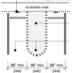
**96" min. width access aisle**, level (max. slope 1:50 in all directions), located beside the van parking space
